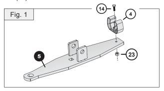
NOTE: After this point, do NOT tighten bolts fully until **Step 7**. You will need the ability to shift parts a little during the assembly.
